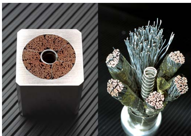
Fig.1 - Multi-wire LTS for nuclear fusion facilities (ENEA, Italy)
